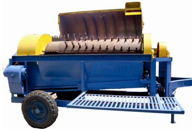
Figure 2. Exploded photograph of developed of Pusa Basmati Rice thresher
